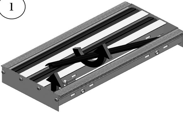
Remove the first deflector by turning and pushing it
