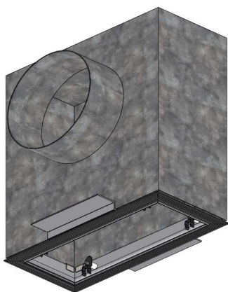
3 - Insert the plenum flush inside the groove formed by the frame and the installation bayonet
