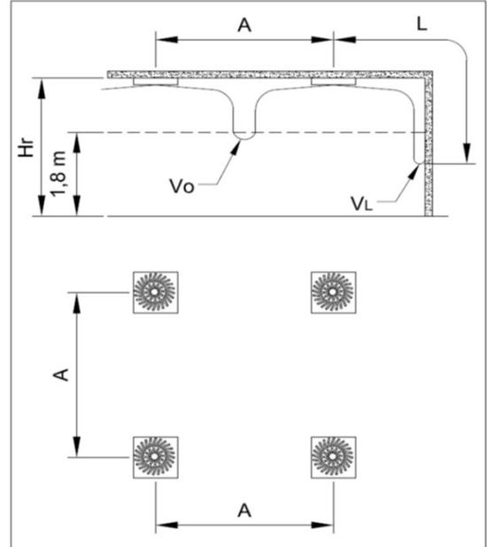
**Dati misurati operando in condizioni isotermiche in accordo con la norma internazionale: ISO 5219 1984: Air distribution and air diffusion - Laboratory. Aerodynamic testing and rating of air terminal devices.**
