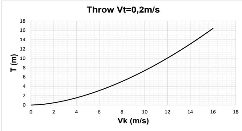
Data measured in isothermal conditions working according to international standard:
