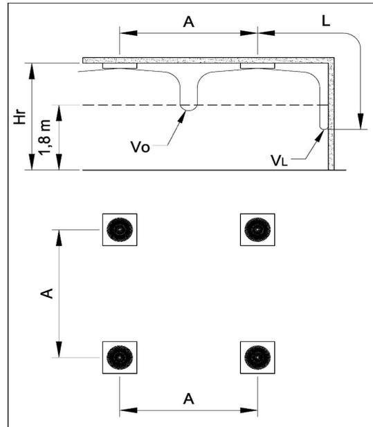
Dati misurati operando in condizioni isoterme in accordo con la norma internazionale: ISO 5219 1984: *Air distribution and air diffusion - Laboratory. Aerodynamic testing and rating of air terminal devices.*
