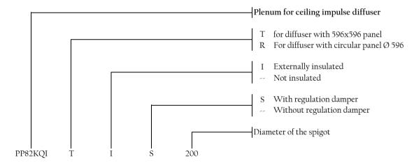
for correct operation, the air inlet diameter of the plenum must be the same of the nominal size of the diffuser
