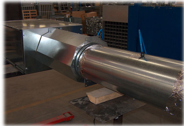
Test of the tight of the casing
